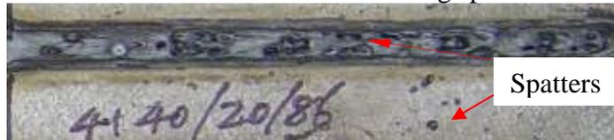
(h) Top view of laser weld at welding speed of 20 mm/s
