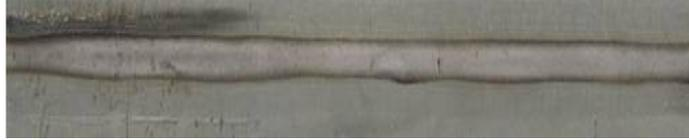
(i) Backside view of laser weld at welding speed of 20 mm/s
