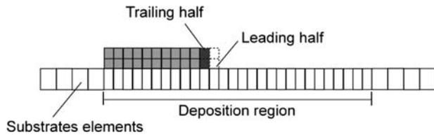
Fig. 3., Finite element model for the LPD process.
