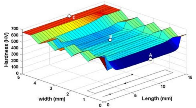
Fig. 5., Surface hardness topography of long-bead pattern.
