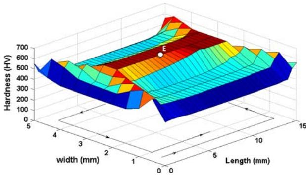
Fig. 7., Surface hardness topography of spiral-in pattern.
