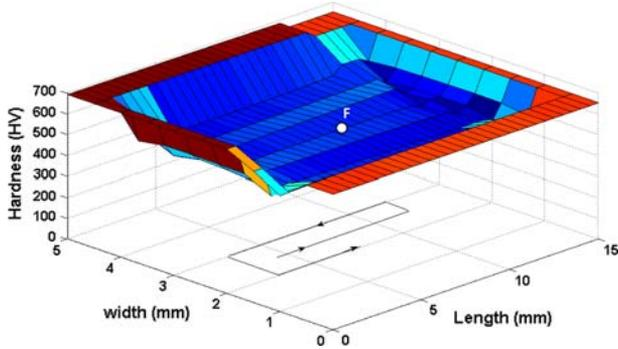
Fig. 8., Surface hardness topography for spiral-out pattern.
