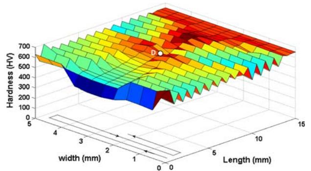
Fig. 6., Surface hardness topography of short-bead pattern.
