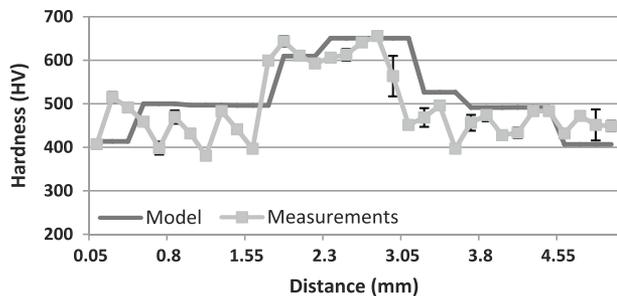
Fig. 14., Measured and predicted hardness along the central traverse line for spiral-in pattern.
