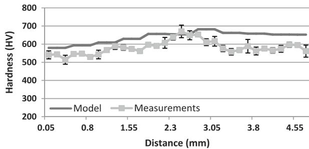
Fig. 13., Measured and predicted hardness along the central traverse line for short-bead pattern.
