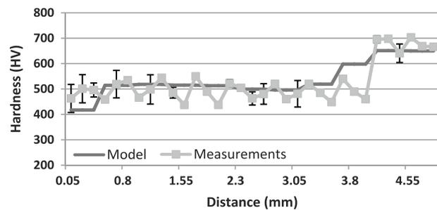
Fig. 12, Measured and predicted hardness along the central traverse line for long-bead pattern.
