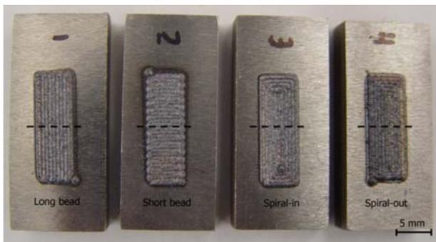
Fig. 11, Experiments performed under different deposition paths.
