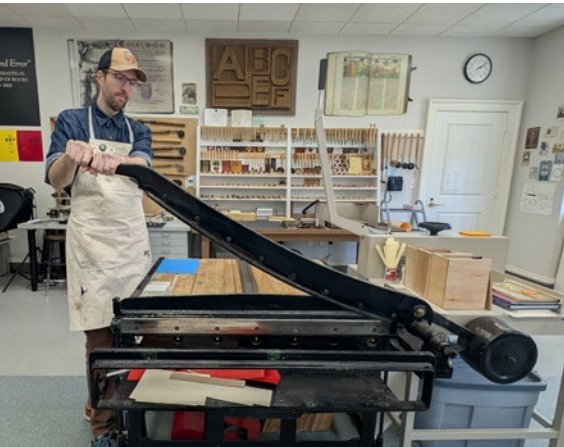
Above Jesse Hunt uses a board shear to cut book board. Right Visitors are often intrigued by the “sci-fi” look of the humidification chamber, which is used to help soften and flatten brittle materials.
