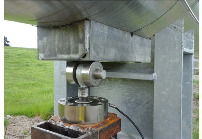
LC Sensor installed on sliding pipe shoe >
