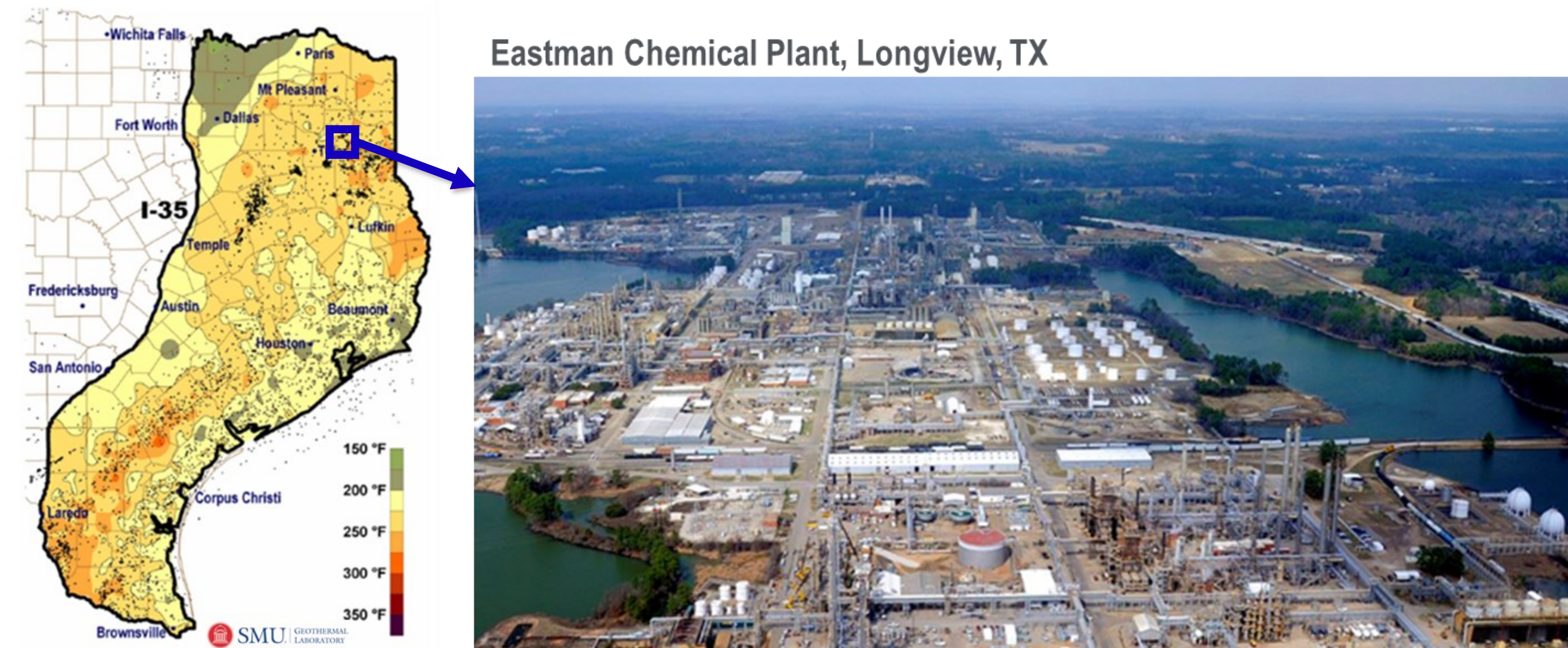
Figure 1. Sub-surface temperature of East and South-Central Texas at 9,000 feet depth (Blackwell, et al., 2010). The study area highlighted with the blue square has regionally high temperatures, but more data points are being added as part of this project to increase the resolution of the heat flow and temperature-vs-depth maps.
