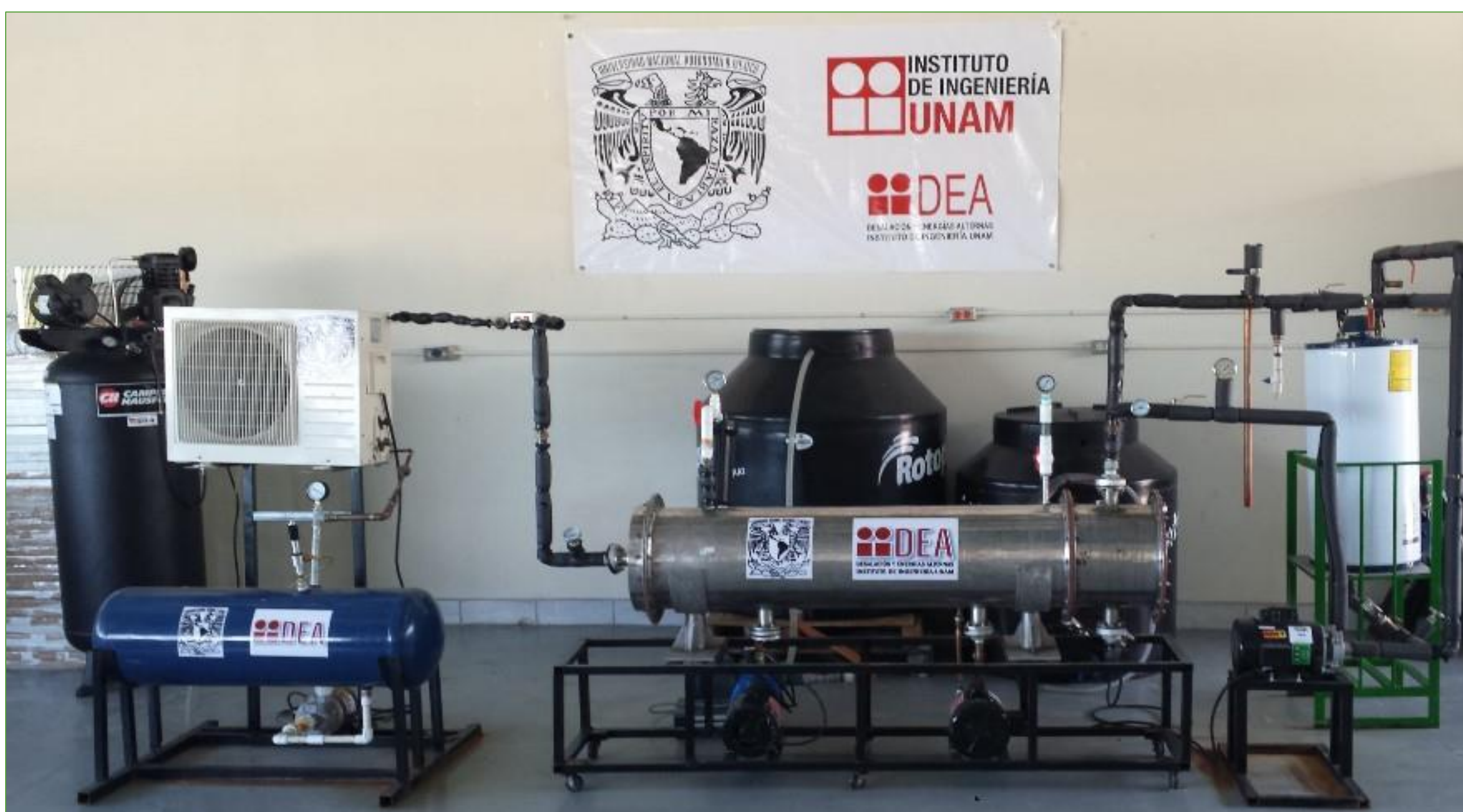
Prototype of the first desalination chamber for experimental purposes, launched in the Polytechnic University of Baja California (UPBC), Mexicali BC.
