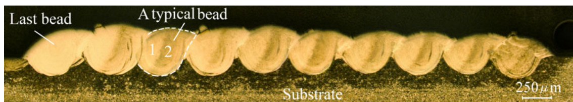
Fig. 16—Cross section of one-section pattern showing regions 1 and 2 in a typical bead.
