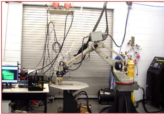
Fig. 3. Experimental setup of laser heat treatment.
