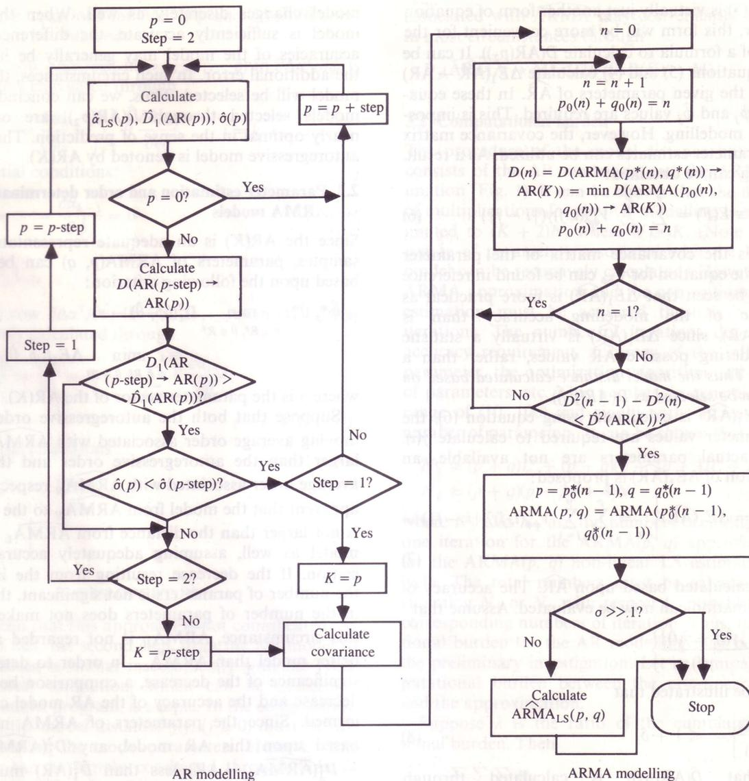
Fig. 1 Identification procedure of ARMA models from large samples
