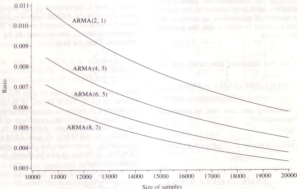
Fig. 2 Ratio of cumulated computational burden versus sample size
