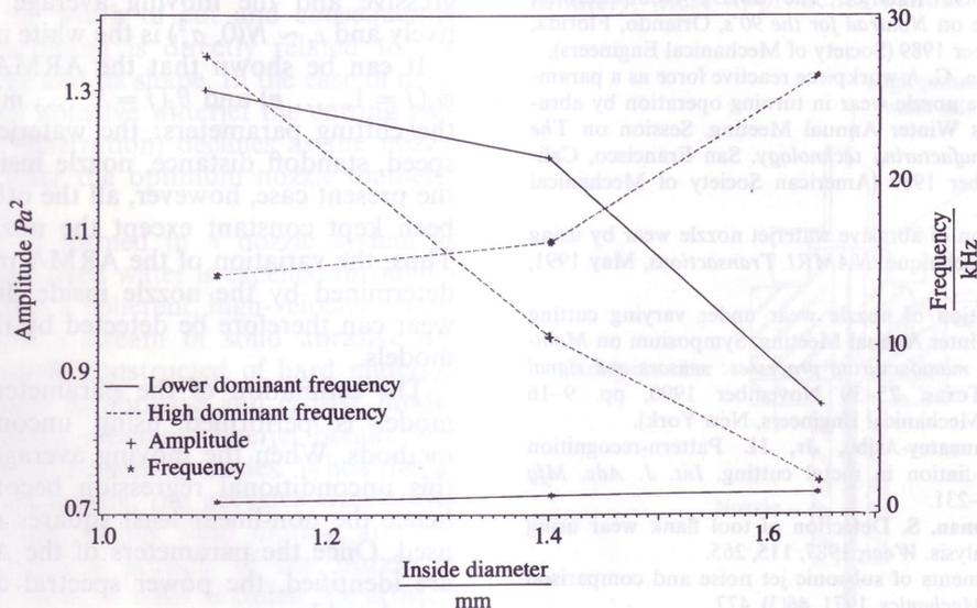
Fig. 6 Two dominant frequencies and amplitudes versus nozzle inside diameters
