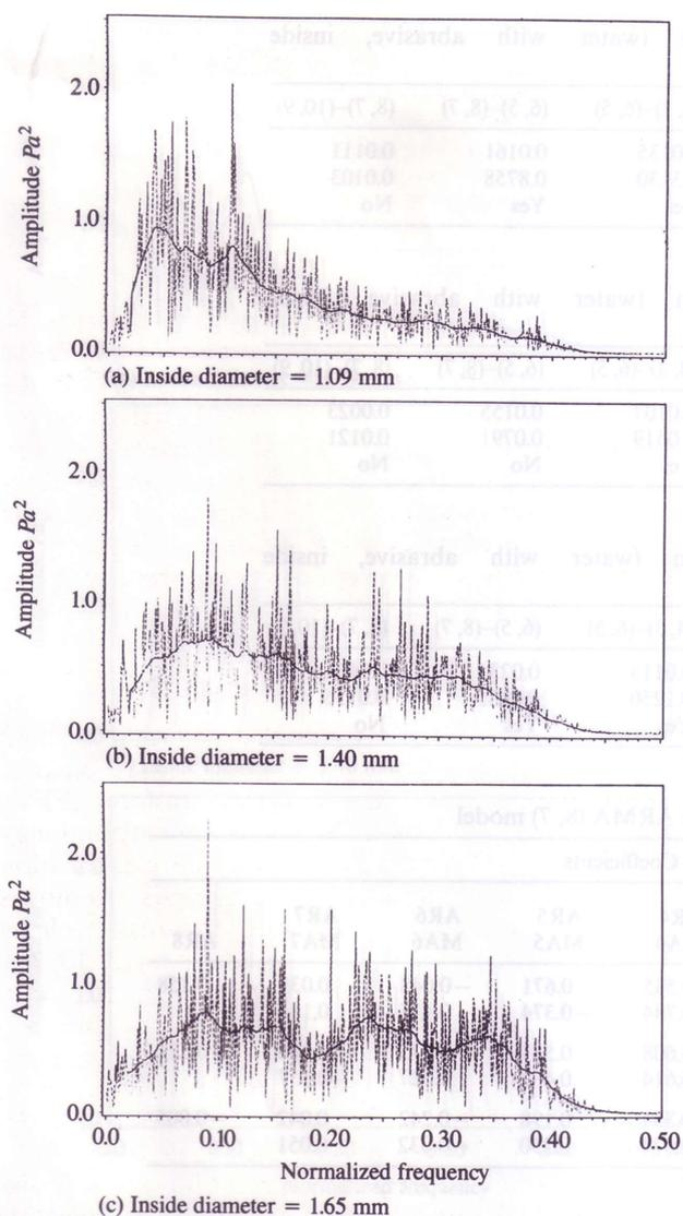
Fig. 4 Comparative power spectrum signal for water and abrasive with smoothing filter and without smoothing filter ( $d = 305$  mm, aluminium oxide)
