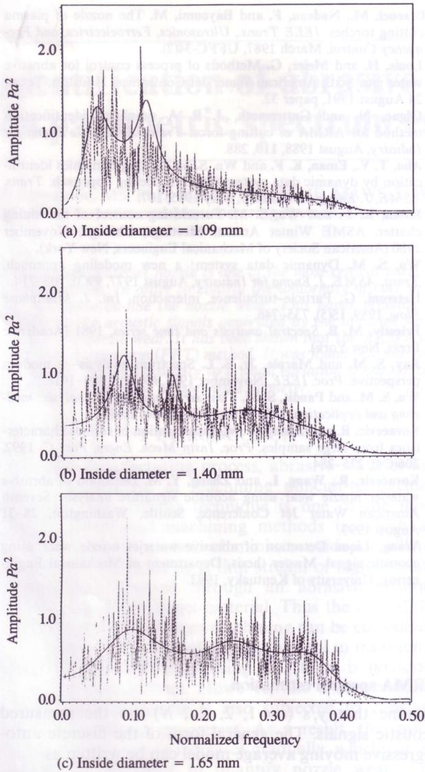
Fig. 5 Comparative power spectrum of acoustic signal for water and abrasive with conventional method and ARMA model method ( $d = 305$  mm, aluminium oxide)
