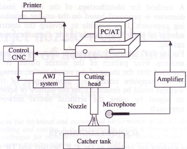
Fig. 7 A closed-loop control system for nozzle wear
