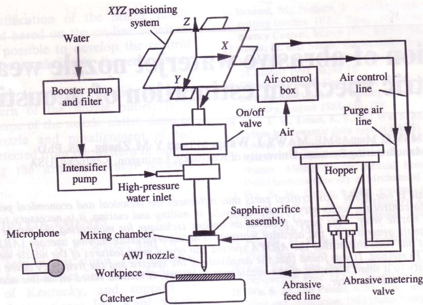
Fig. 2 A general concept of abrasive waterjet cutting system
