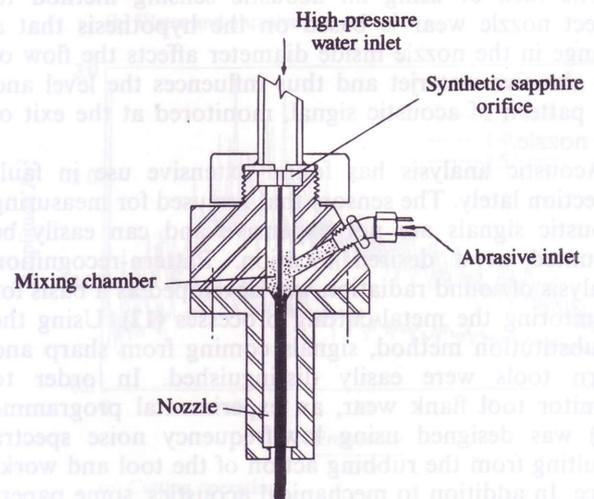
Fig. 1 Schematic presentation of abrasive waterjet cutting head
