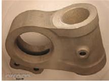
**Figure 4. 3D component built by the electron beam process. (Photo provided courtesy of ARCAM AB)**
