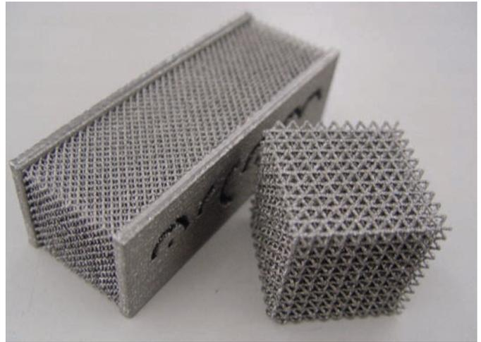
**Figure 6. Lattice structures built of Ti-6Al-4V by the electron beam process.**
