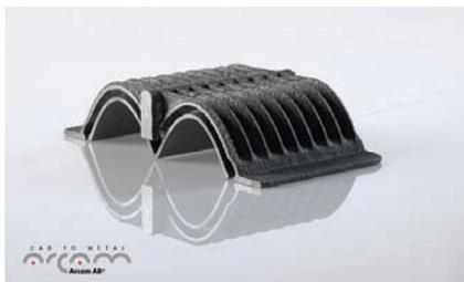
**Figure 1. Component with 3D cooling channels built of Ti-6Al-4V powder by the electron beam process. (Photo provided courtesy of ARCAM AB) [1]**
