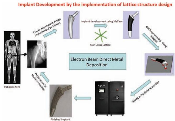
**Figure 7. Application of electron beam system in building medical models and implants.**
