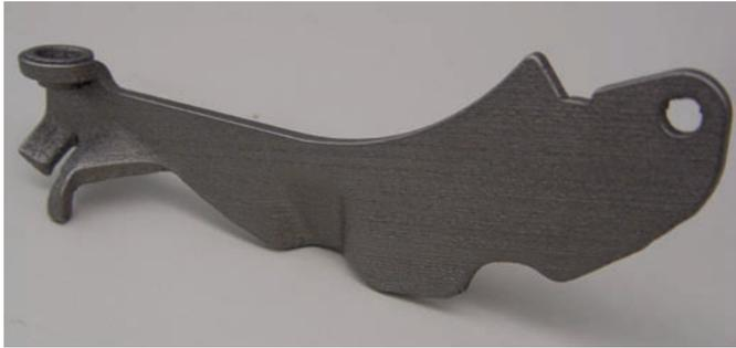
**Figure 5. 3D component built of Ti-6Al-4V by the electron beam process.**
