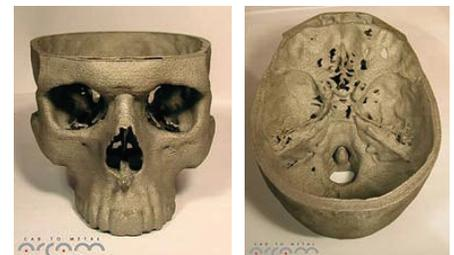
**Figure 3. A skull built of cobalt chromium alloy by the electron beam process. (Photo provided courtesy of ARCAM AB) [1]**
