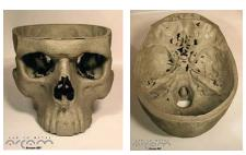
Figure 3. A skull built of cobalt chromium alloy by the electron beam process. (Photo provided courtesy of ARCAM AB) [1]
