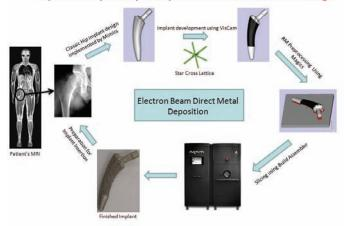
Figure 7. Application of electron beam system in building medical models and implants.
