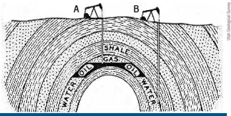
In a "classic" formation, geothermal water may be found along with oil and gas. To enhance oil or gas recovery from Well A, water or other fluid or gas can be pumped down the deeper Well B. For geothermal energy production, hot water can be pumped up from Well B and the spent water reinjected in Well A to keep the reservoir productive.
