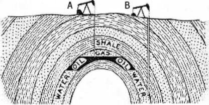
In converting to geothermal energy production, hot water can be pumped up from Well B and the used water reinjected into Well A to keep the reservoir productive.
