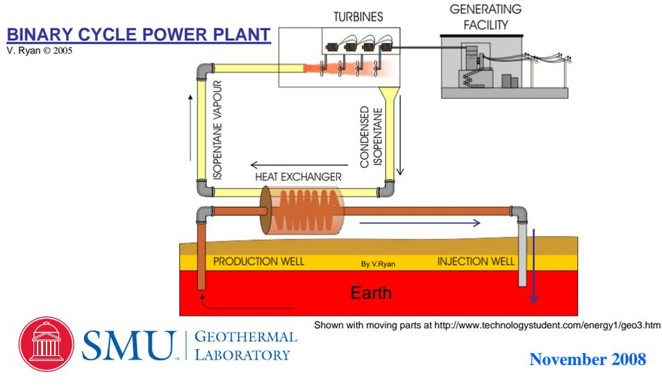
There are different types of geothermal power plants. For places where the water is less than 300°F, a binary power plant is used. Most small geothermal power plants (less than 10 MW) are binary geothermal power plants.
