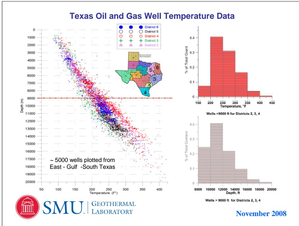
To develop geothermal energy in Texas, the fluid temperatures need to be at least 200°F. Remember that the hotter the better so the wells with temperatures over 300°F are the first locations to look into for a geothermal power project. As you can see, below about 9000 feet in eastern - southern Texas the temperatures are usually above the 200°F starting point. Most of the wells are located between 10,000 and 13,000 feet that are above 200°F.
