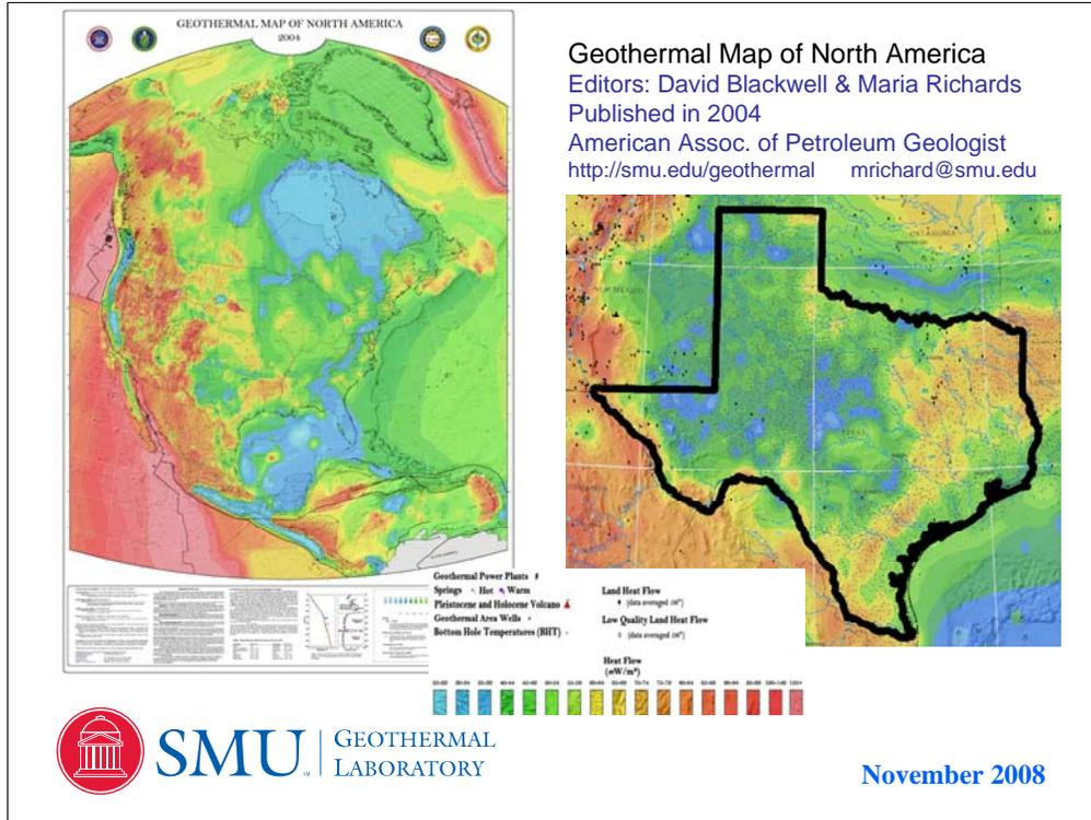
In the production of the Geothermal Map of North America, Dr. David Blackwell incorporated the data from oil and gas wells. Reviewing the temperature data from 10,000s of oil and gas wells, it became apparent that they reemphasized the existing heat flow data base. Where the heat flow is higher than expected, temperatures from the oil and gas wells were higher as well, and vice versa for colder locations.
