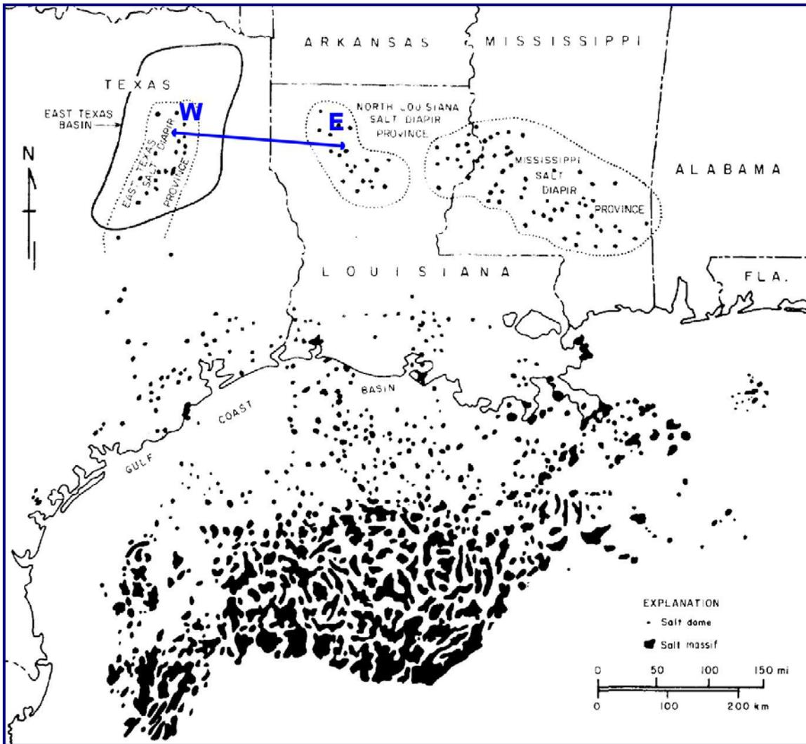
Figure 6. Map of East Texas basin, location of inland salt-diapir provinces, and salt domes, (Seni and Jackson, 1983). Cross-section in Figure 5 is shown as a blue line.
