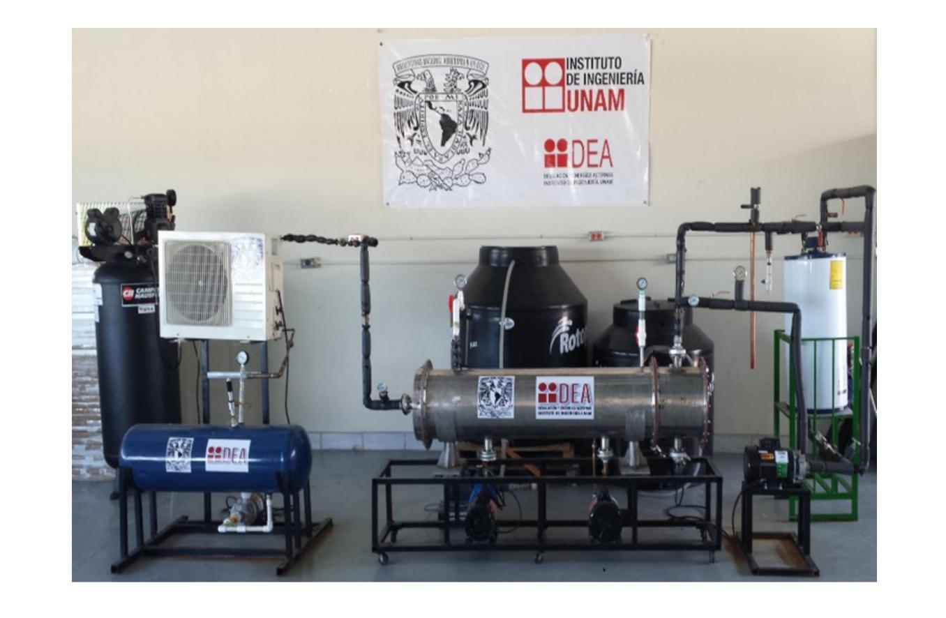
Prototype of Modular Geothermal Desalination Unit
