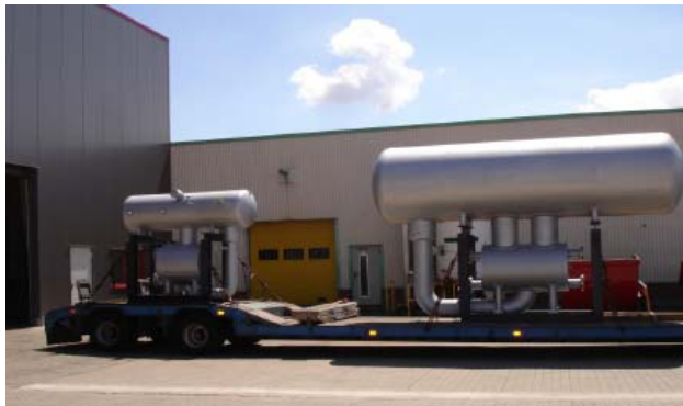
Low temp flooded evaporator for climatic test chamber in auto industry (BMW)
