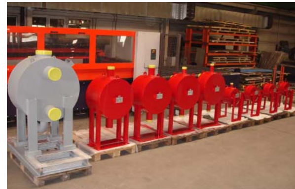
Condensers & Evaporators for Ice Rink in Switzerland
