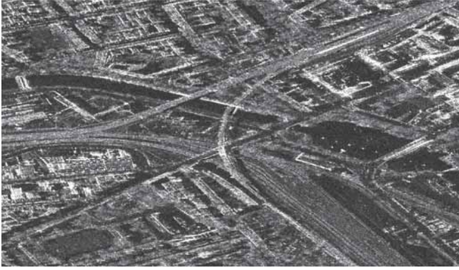
Fig. 1. High-resolution spotlight SAR amplitude image of the Eisenbahn bridge in Berlin acquired by a TerraSAR-X satellite sensor.
