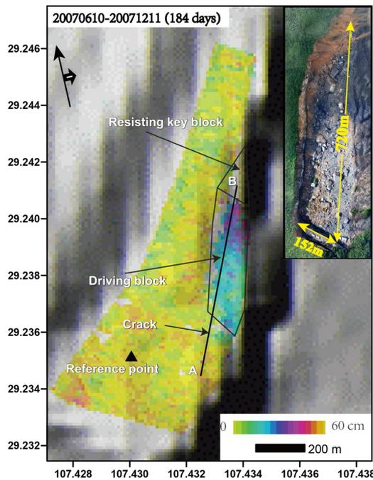
**Fig. 6.** The cumulative deformation map during 10 June and 11 December 2007 (184 days). Resisting key block, driving block and one of the back cracks of the Jiweishan slide are outlined. Black triangle indicates the reference point for InSAR time-series analysis. Profile AB will be discussed in Fig. 7. The inset is the aerial photograph taken after Jiweishan sliding (Yin et al., 2011).
