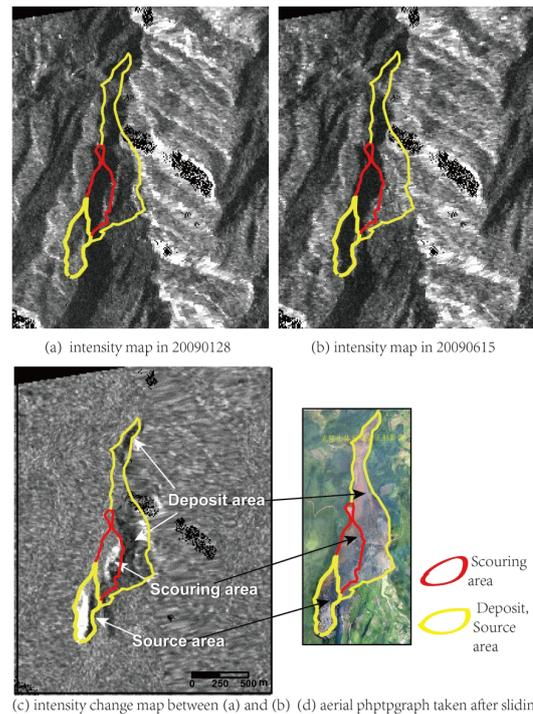
**Fig. 8.** Two SAR Intensity images acquired on 28 January 2009 (a) and 15 June 2009 (b). (c) Intensity change map between (a) and (b). Dashed polygon is superimposed on each map onto indicate the affected area inferred from (d) aerial photograph taken after sliding. In (c) and (d), source area, scouring area and deposit area are all indicated.
