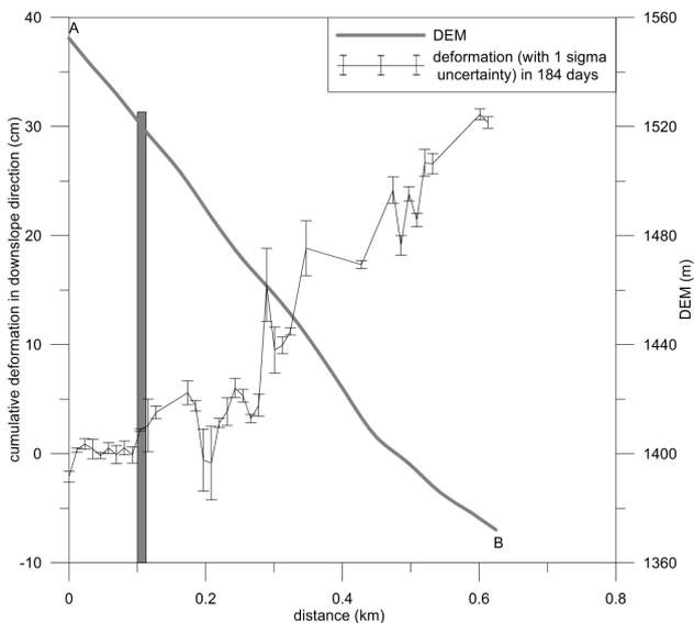
**Fig. 7.** Cumulative deformation in down-slope direction within 184 days and SRTM DEM along profile AB shown in Fig. 6. 1-sigma uncertainty indicates the InSAR deformation accuracy in down-slope direction. The vertical grey bar indicates the back crack point (shown in Fig. 6).
