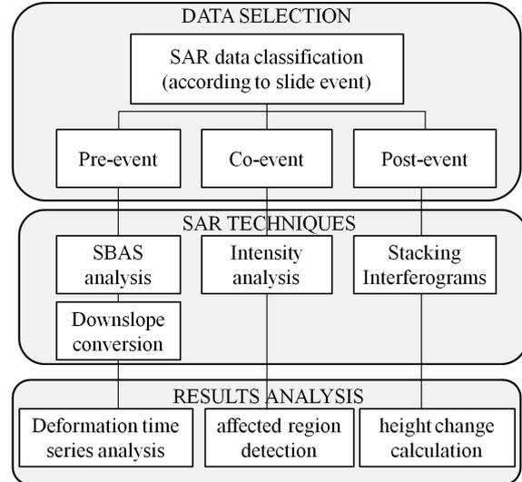
**Fig. 3.** The flow chart of SAR analysis for pre-, co-, and post-slide analysis.
