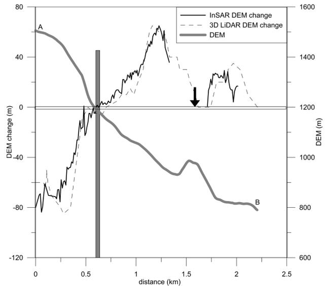
**Fig. 10.** Cross section of pre-slide SRTM DEM, DEM change measured by InSAR and 3-D lidar techniques after Jiweishan sliding along profile AB. The vertical grey bar indicates the transition point between the source area and the deposit area, while the black arrow shows the location of scouring area between two deposit areas.
