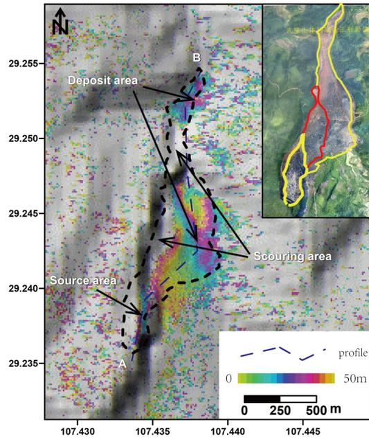
**Fig. 9.** DEM change map calculated by InSAR stacking method after Jiweishan sliding. The black dashed line delineates the affected region based on an aerial photo and the blue dashed line represents the location of the profile AB shown in Fig. 10.
