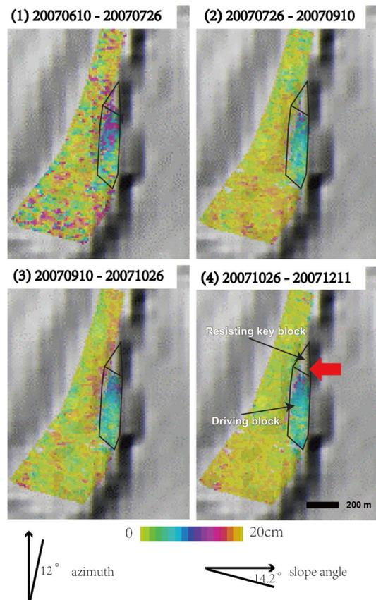
**Fig. 5.** Deformation maps within 46 days over the Jiweishan region before the 5 June 2009 slide, the red arrow indicates the same location as shown in Fig. 4. The slide geometry is shown at the bottom of the figure.
