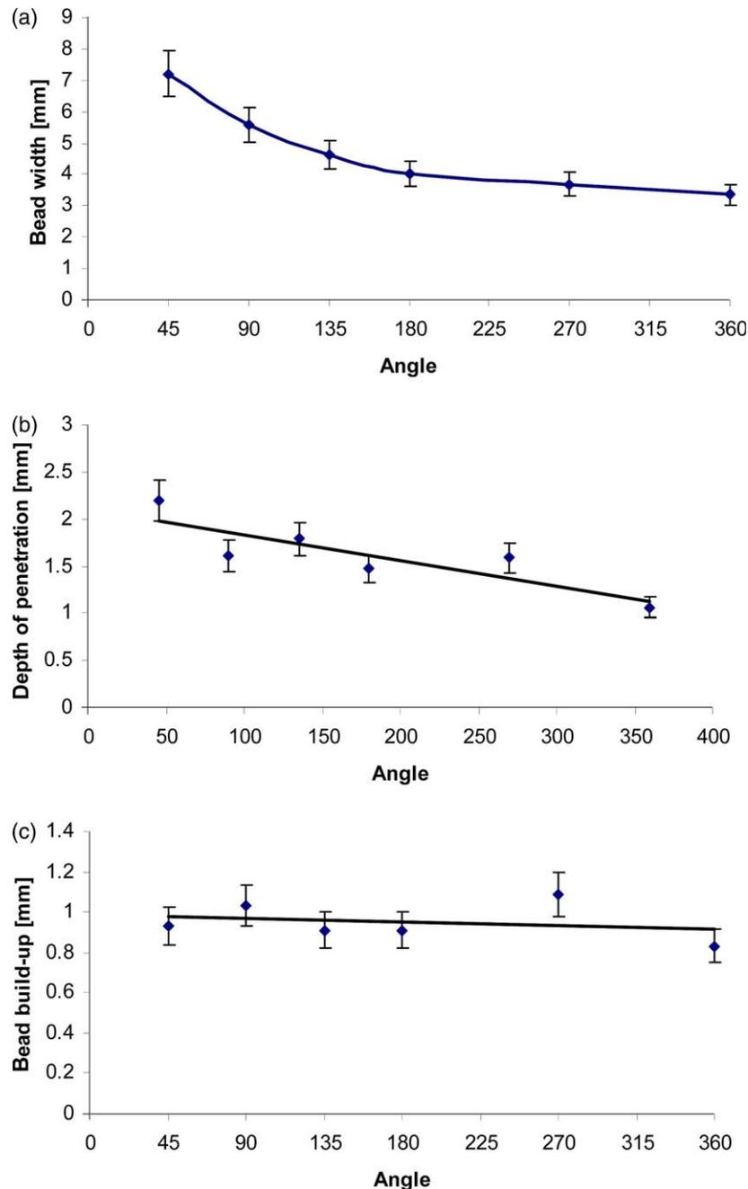
Fig. 5. (a–c) Influence of the geometry on the bead. (a), Bead width; (b), depth of penetration; (c) bead build-up.
