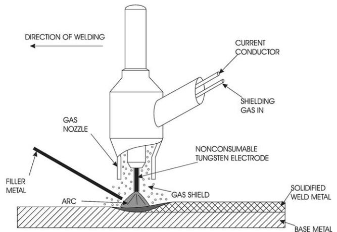
Fig. 2. Gas tungsten arc welding process.
