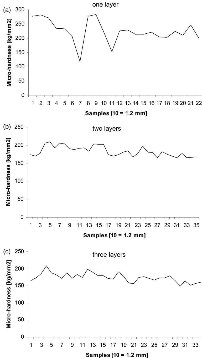
Fig. 14. Microhardness of deposited layers.
