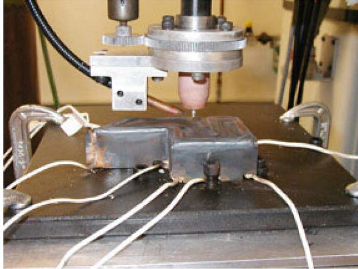
Fig. 6. Embedded thermocouples.
