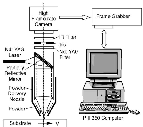
Fig. 4 Infrared image acquisition system
