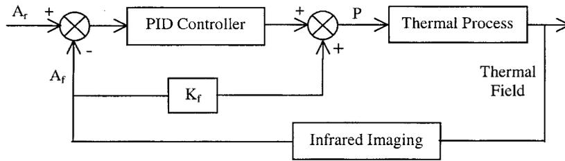
Fig. 8 Schematic diagram of the closed-loop control system
