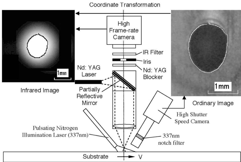
Fig. 7 Molten pool edge determination for infrared image
