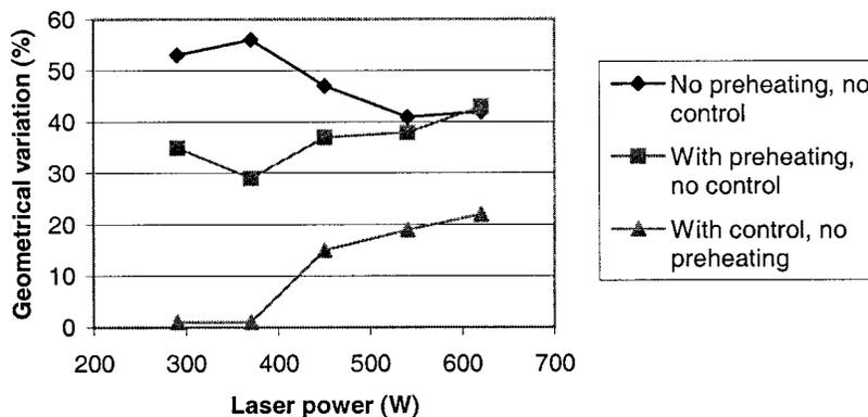
Fig. 14 Comparison of geometrical variation of laser cladding results
