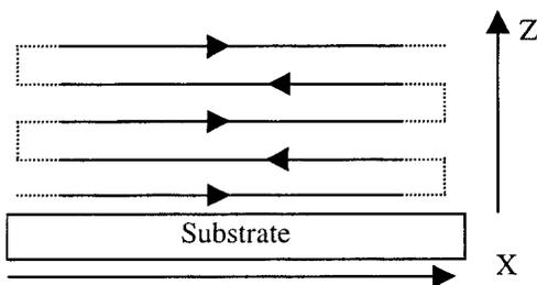
Fig. 9 Scanning path for single-bead wall building
