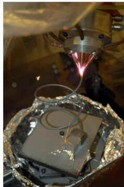
An example of multiaxial deposition on the MultiFab system
