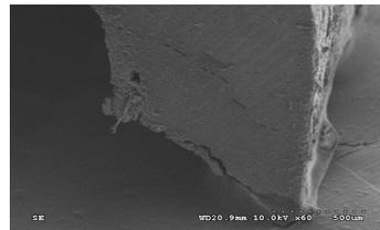
**Cracking pattern in rabbit femur bone compression tested at strain rate of 225 s<sup>-1</sup>**
