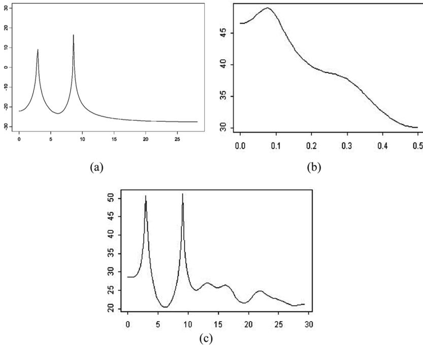
**Figure 6.** (a)  $M$ -spectral density estimator based on the Euler(4, 4) model; (b) AR(4)-spectral density; (c)  $M$ -spectral density based on Euler(14) model.
