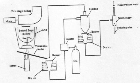
Fig. 6 Ice particle injection ice jet machining
