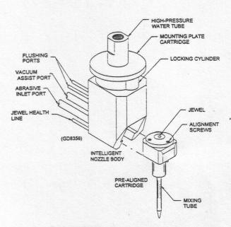
Fig. 5 Schematic of quick change nozzle
