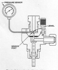
Fig. 4 Schematic of orifice health sensor
