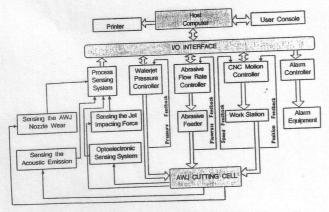
Fig. 7 Block diagram of new generation of AWJ cutting system
