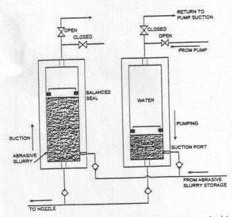
Fig. 3 Schematics of high pressure continuous abrasive suspension jet
