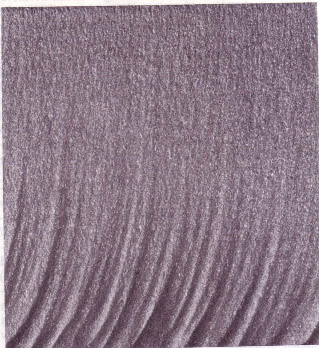
Fig. 2 Striation formation during abrasive water jet machining (sample: aluminium)
