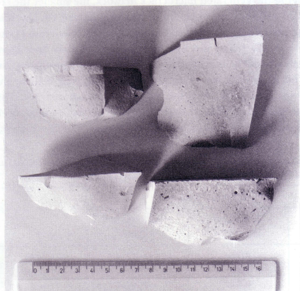
Fig. 10—Photograph of wear debris of plain cement matrix subjected to high speed water flow (scale in mm).
