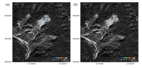
**Figure 9.** TerraSAR-X intensity change between 2017 and 2018 (a) and between 2018 and 2019 (b) in the Gold Basin landslide. Cool color indicates intensity decrease and warm color intensity decrease [57].
