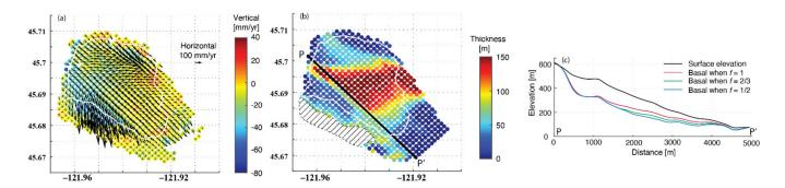
**Figure 6.** (a) Displacement velocity maps of Crescent Lake landslide. (b) Landslide thickness with rheology parameter f = 2/3. (c) Profiles of surface elevation and landslide basal surface elevations with different rheology parameters along the transect P-P' shown in (b) [46].
