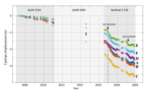
**Figure 8.** Long-term deformation of the Hooskanaden landslide from 2007 to 2019. Cumulative along-slope displacements of multiple points (cyan dots in Figure 7) of the Hooskanaden landslide [83].
