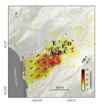
**Figure 7.** Three-dimensional displacement field of the February 2019 movement of the Hooskanaden landslide reconstructed from Sentinel-1/Sentinel-2 pixel offset tracking [83].
