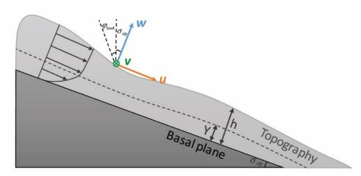
**Figure 1.** The configuration of landslide body. The landslide basal topography is modeled as a plane that defines the coordinates for the horizontal motion vector u and v of the slide and the vertical motion vector w. The thickness of landslide h goes through the lower yield zone and the overlying plug region: in the yield zone, the materials deform viscously with zero velocity at the basal plane; in the plug region, the materials move uniformly as a plug with no shear strain.
