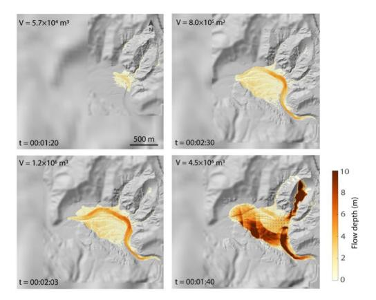
**Figure 10.** Maximum inundation zone of the campground as  $m_0 - m_{crit} = -0.02$  meaning that landslide body is highly mobile ( $m_0$  and  $m_{crit}$  are initial and critical solid volume fraction of sediment). V denotes volumes ranging from  $5.7 \times 10^4$  to  $4.5 \times 10^6$  m<sup>3</sup>, and t is timestamp [57].
