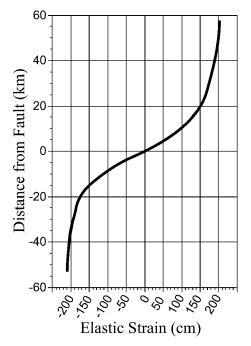
Figure 5. Reconstruction of elastic deformation for area north and south of North Anatolian fault just prior to Kocaeli earthquake, based on profile shown in Figure 3 but adjusted for radar look. This line is equivalent to datum  $D_i$ , in Figure 4C, just prior to rupture, and two other lines represent datum  $D_i$ , in Figure 4C, just after faulting.
