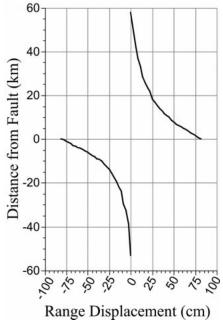
Figure 3. Range displacements measured on interferogram, north and south of North Anatolian fault. Maximum range displacement on this profile was about 2.1 m on either side, or total fault displacement of 4.2 m. Displacement continues for nearly 60 km on either side of fault at its maximum, although only ~50 km is recorded in this profile. Note that several fringes could not be resolved near fault and within body of water (dark area above Gölcük in Fig. 2).
