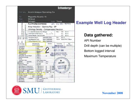
From the Texas Railroad Commission, oil and gas well logs can be downloaded, or copies can be made through the UT Austin Bureau of Economic Geology Well Log Library. The top page of a well log is named a header. From the header it gives basic information about drilling the well and the parameters of the new well.
