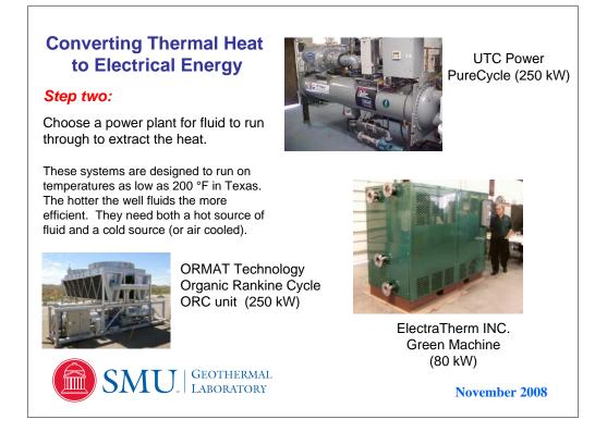
What is exciting about this slide, is that there are more and more binary technologies being developed. In 2004, when the Geothermal Map of North America was being produced, no one was making small (less than 1 MW) power plants. ORMAT Technologies had made some in the past, but were not focusing on making them at the time.
