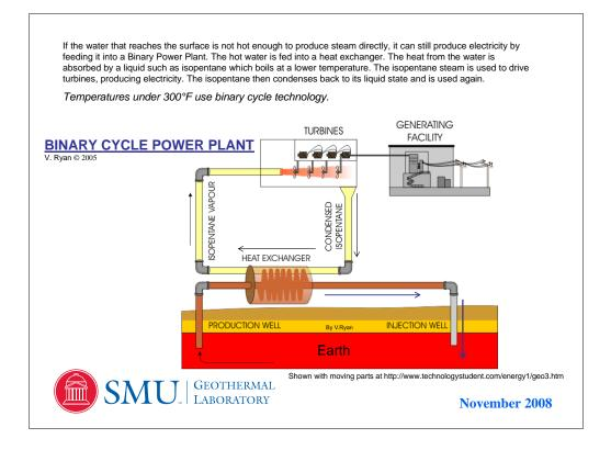
There are different types of geothermal power plants. For places where the water is less than 300°F, a binary power plant is used. Most small geothermal power plants (less than 10 MW) are binary geothermal power plants.
